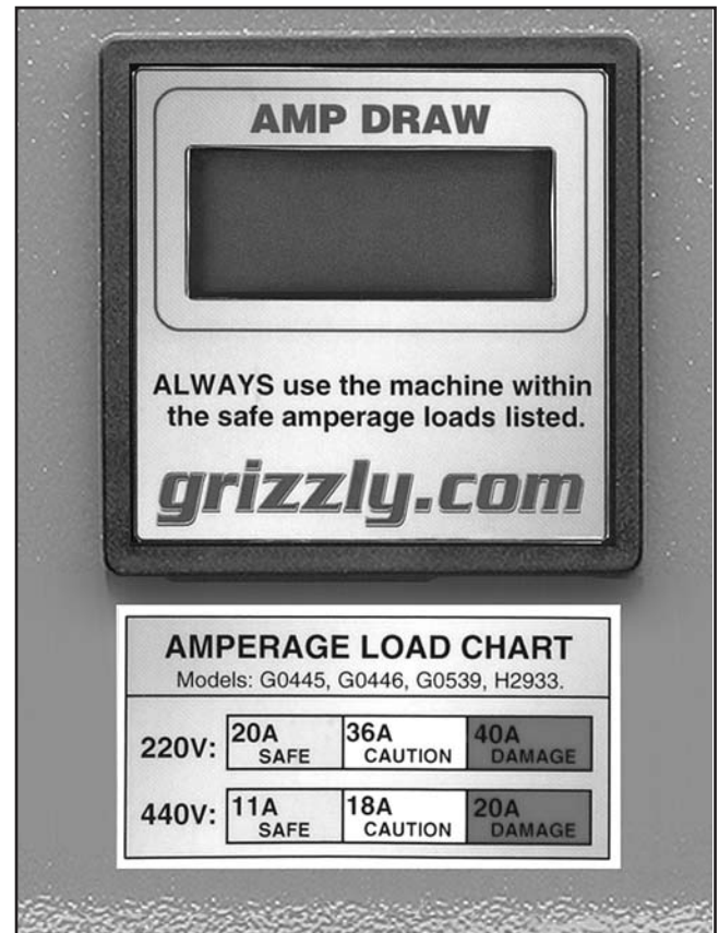
Figure 16. Typical amp draw meter and load chart.
